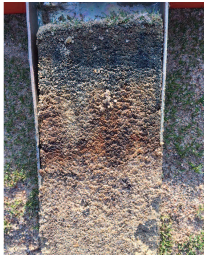
An example of a black layer problem and why there is a need for chemical and physical aeration.
